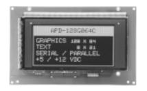
The APD-128G064C is a dot matrix graphic display with an array of 128 x 64 pixels available. The module is composed of a highly reliable DC plasma display, ASCII input graphics controller, DC converter and drive circuitry which are assembled to form a rugged, slim profile display sub-system.
